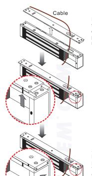
Fasten the mounting plate on the site then install electromagnet lock with power lead cable through mounting plate slot hole.
